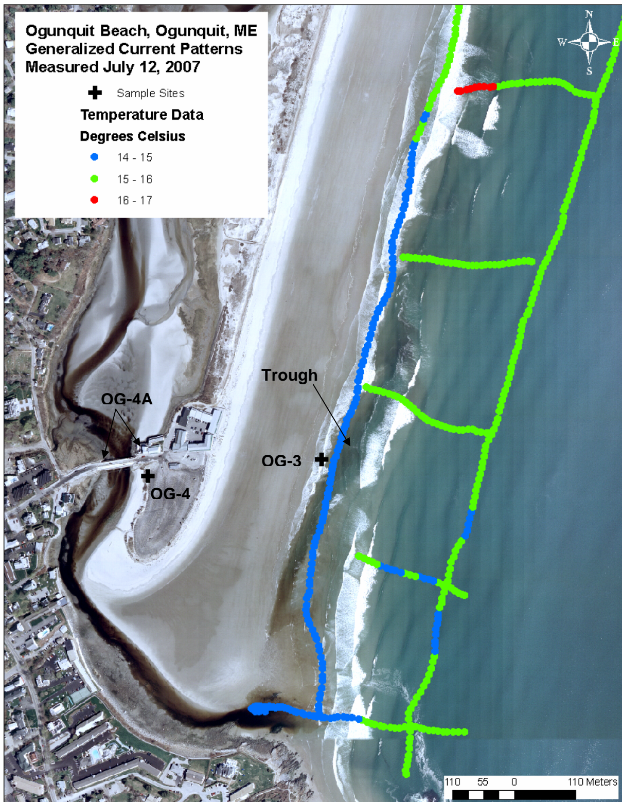
Figure 9. Temperatures recorded by MGS (Slovinsky and Dickson, 2008) during the July 2007 ADP survey show a distinct cooler water mass that is located within a trough that is parallel to the beach, in relation to the locations of OG-3 and OG-4. The potential locations for OG-4A are also shown. Base image from MEGIS (2003).
