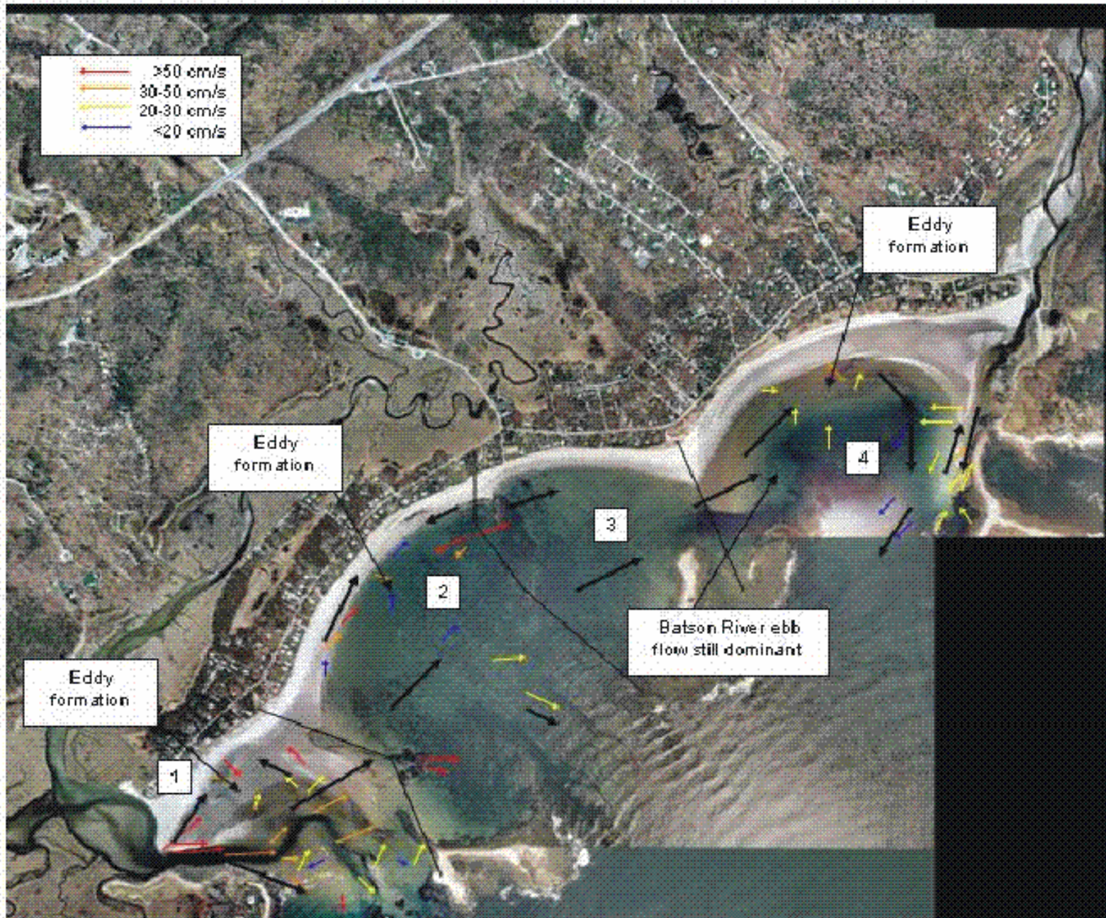
Figure 3. Generalized results of MGS ADCP current study conducted on August 19, 2005 during ebb tidal conditions at start of spring tidal cycle. Black arrows indicate general flow pattern, while colored arrows indicate actual data (see legend for speeds). Study area was divided into 4 littoral cells (labeled 1-4) based on current patterns and morphologic characteristics. 50 cm/s is approximately half a nautical mile per hour. Photograph from MEGIS.
